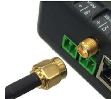
2. Before you mount the T4000 you will need to test the signal strength in your chosen location. If the signal strength is poor you will need to install a high gain antenna or find a more suitable location for the T4000 in order to obtain greater signal strength.
